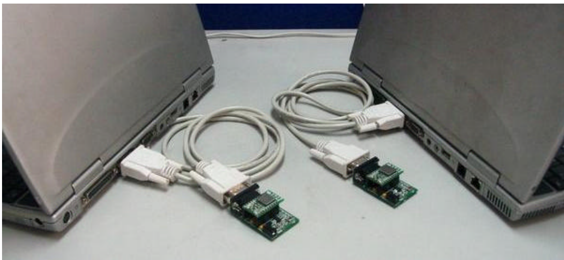
Figure 2 The two device connect embedded module respectively, the function is equal to one serial cable.
